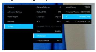
2. Another way to find the Camera IP address (On same Subnet) is to use the AVer IPCam Utility to find the camera. AVer software can be found here:
