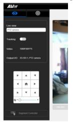
6. Next, select the settings gearbox then select *Video & Audio setting*, this is where you can select Video Output, Audio, and the type of Streaming mode to use and Streaming video standard. \*Note: This *IP Streaming Mode* is used for RTSP and RTMP Streaming.
