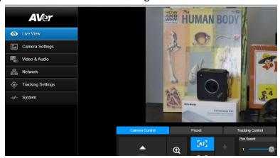
4. Next, after selecting the *Video & Audio* setting, verify the Video Mode you are in. In this setup you should *NOT* be in NDI and *Stream Only* Video Mode, as it will disable the USB output.
