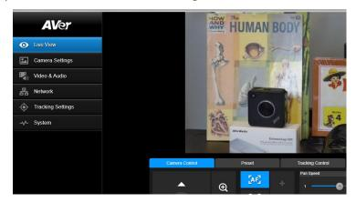
Next, after selecting the *Video & Audio* setting, verify that you have either "Stream Only" selected or "USB + Streaming" selected. Select your Stream Video Output, Bitrate, Framerate, Encoding, etc.
