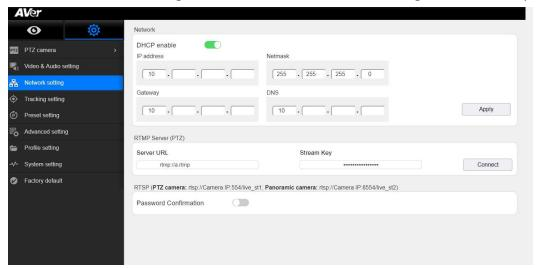
8. Next, notice the RTMP Server URL selection, this is where you will "paste" the URL string from Microsoft Stream as well as the Stream Key from Microsoft Stream. \*Note: The RTMP Stream will use the PTZ IP Stream Mode output configuration.
