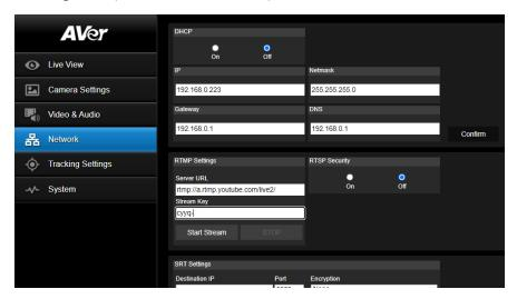
\*Note: Once streaming has started do not change the Stream Video Output on the fly, you will need to "Stop" streaming, change the Stream Video Output, then "Start" the stream again.
